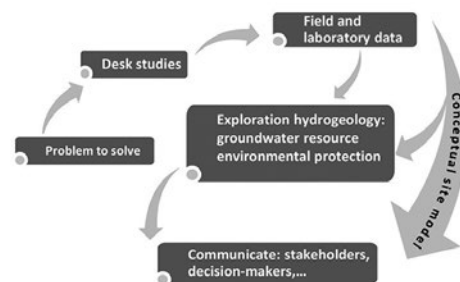
Figure 2: Conceptual site model: a flow path for an integrated exploration hydrogeology approach (after Chaminé et al. [37]).
