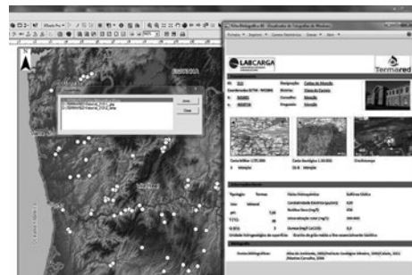
Figure 2: An example of the GIS output for the NW Portugal (adapted from Teixeira et al. [26]): 1. Application tool to create hyperlinks between features (line, point or polygon) and other files; 2. Hyperlink addressed to a file (image or text); 3. Visualisation of photo details for the water inventory; 4. Hydrogeological inventory datasheet (field and desk data); 5. Regional hydrogeological mapping.
