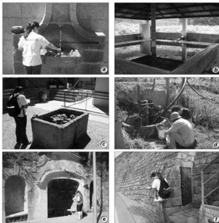
Figure 1: Several aspects of the fieldwork campaigns (Porto and Penafiel urban areas): Measuring temperature, pH and electrical conductivity in a fountain (a); georeferencing public washing places (b and c); measuring the piezometric level in a dug-well (d); georeferencing fountains (e) locating a water mine (f).
